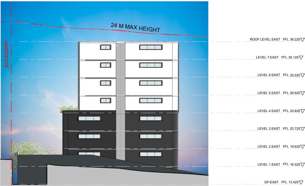
EAST WING NORTH ELEVATION 1 : 200
