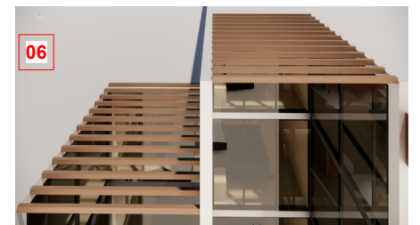
ALUMINIUM SUN LOUVRES, DULUX POWDER COATED STONE BEIGE SCYLLA
