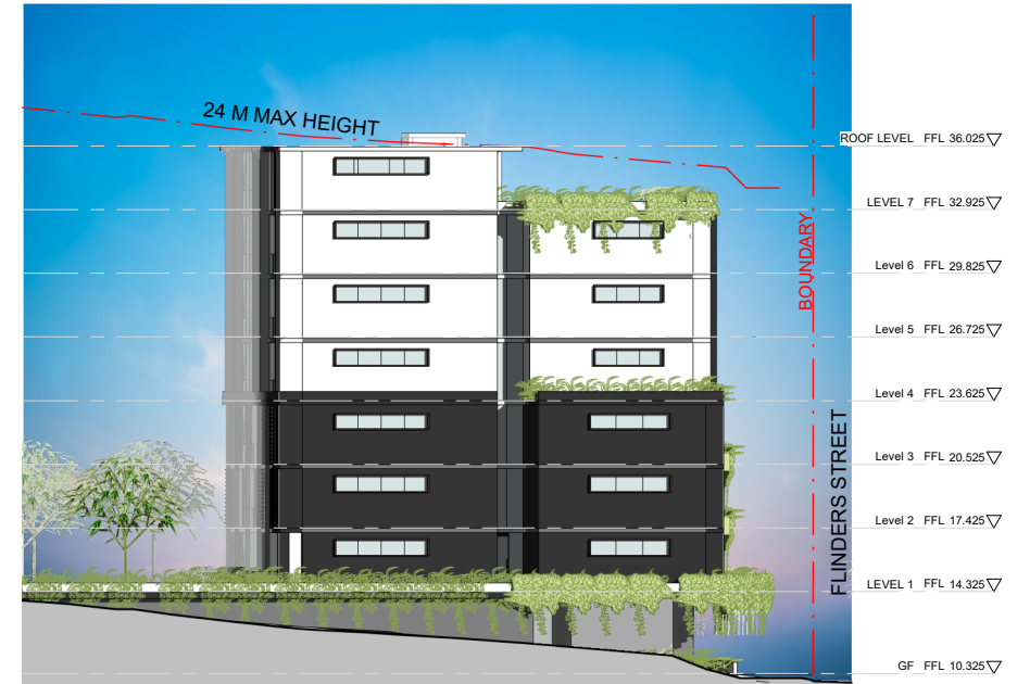
WEST WING NORTH ELEVATION 1 : 200
