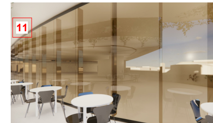
STRUCTURALLY GLAZED STOREFRONT
