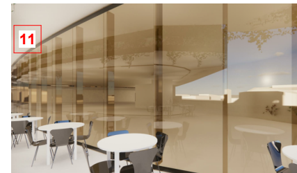
STRUCTURALLY GLAZED STOREFRONT
